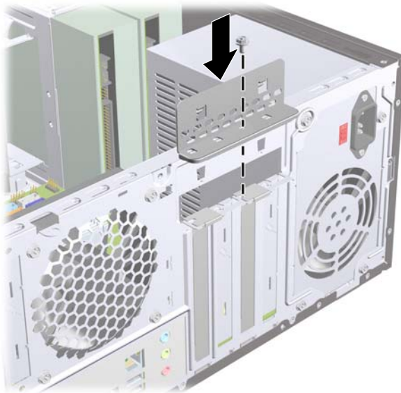
Figure 6-13 Securing the Expansion Cards and Slot Covers
